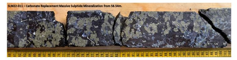
Figure 1: Massive CRD sulphide intercept from Hole SLM22-011 at the Grizzly Ag-Zn-Pb-Cu-Au Target (SLM22-011) showing typical sulphide textures. (Chalcopyrite = Cpy; Galena = Gn; Sphalerite = Sph; Pyrite = Py). This intercept is part of the 1.16m zone grading: 1,145g/t Ag, 23.5% Zn, 23.2% Pb, 0.52% Cu, 0.37g/t Au.
